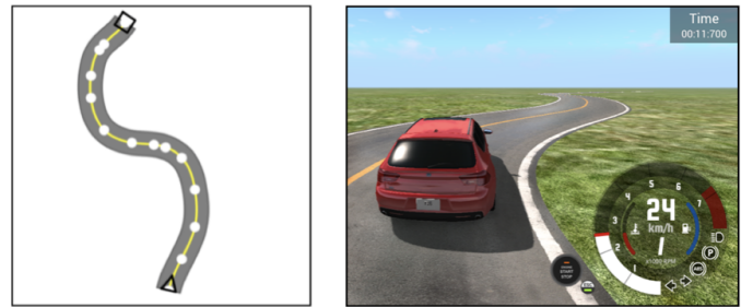
Fig. 1: A driving task for lane keeping assist systems (left); test simulation in BeamNG.tech (right).
